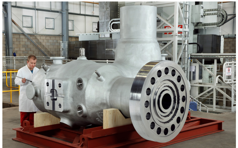
5 off Left Hand & 5 off Right Hand 1000MW casings for the Shenhua Guohua Jiujiang power station, China. These consisted of CrMoV castings issued by Goodwin Steel Castings which were then fabricated to the F91 forgings
