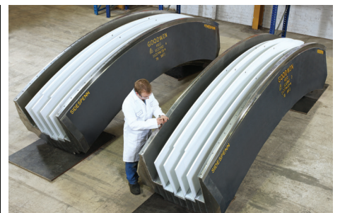
Finished machined splay saddles.
